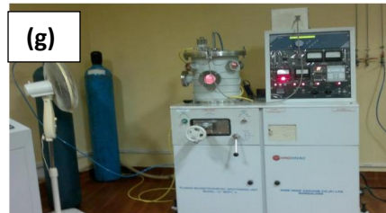
Fig. a. Ferroelectric MOS transistor. b. C-V characteristic of fabricated MFIS capacitor. c. XRD results of deposited PZT film. d. Fabricated MOS capacitors. e. Thermal evaporator for metallization. f. Ellipsometer for thickness measurement. g. Sputtering unit for thin film deposition. h. Furnace for annealing.
